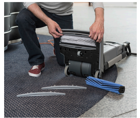
Apart from getting faster cleaning of hard floors, you will also be able to freshen up smaller carpets, including removal of spots, by adding an optional carpet kit. Brush and squeegees can be removed without any tool making daily maintenance operations easy and fast
