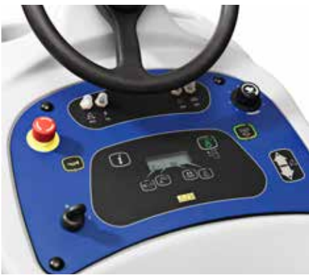
The intuitive dashboard, one touch button and user-friendly menu for operation settings make SC1500 easy to operate even for beginners
