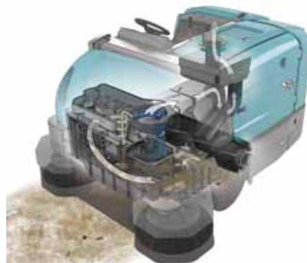
Machines with HEPA filtration system (Option)
