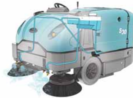
Machine with wet side brush dust control (Option)
