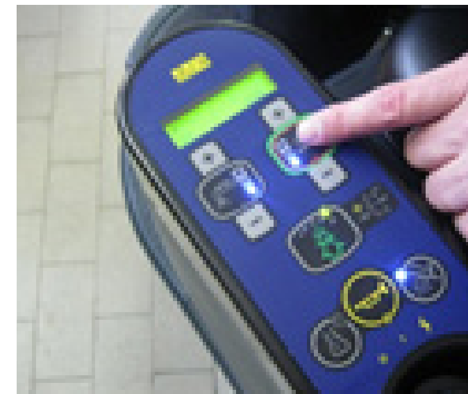
13. Make sure that deck and squeegee are moving down when pressing the button.
