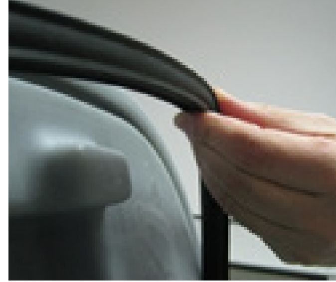
4. Recovery tank seal cover must correctly installed and in good condition.
