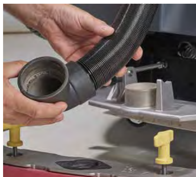
1. Check if the suction hose is correctly installed and cleaned.
