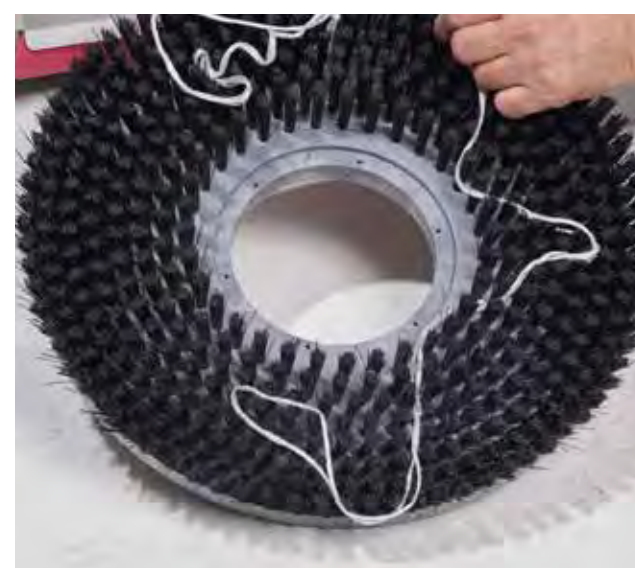
3. Turn brushes counter clockwise and check if there are external materials change avoiding to impeding or prohibiting.
