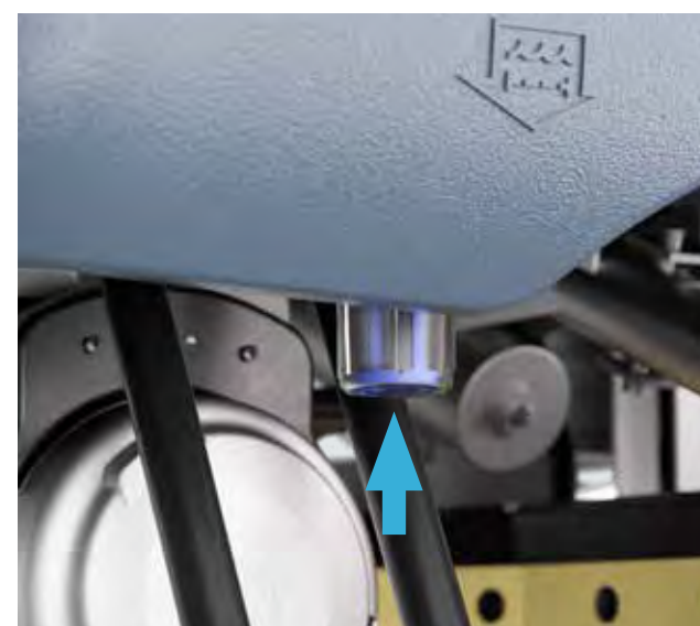
3. Check if the solution filter is cleaned.
