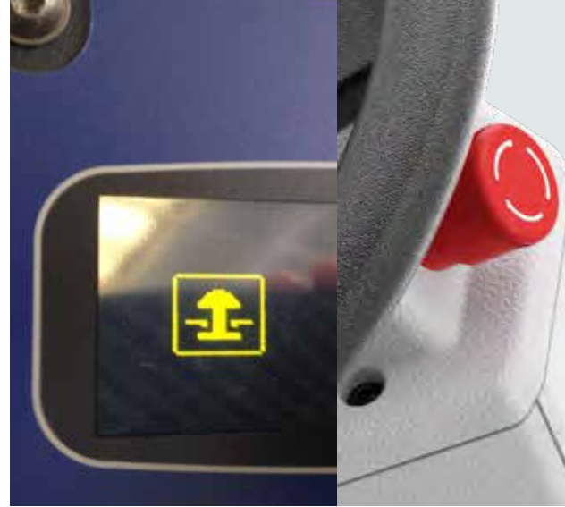
2. E-stop icon appears on display when E-stop switch is engaged. Twist E-stop switch until it pops out to enable machine function.
