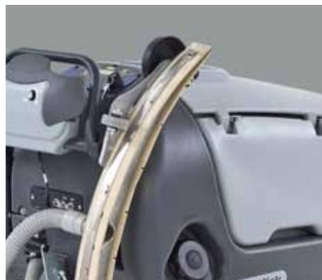
*A built-in squeegee hanger makes transport easier through corridors/ thresholds*
